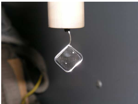
Fig. 3. Tungsten sample installation.
