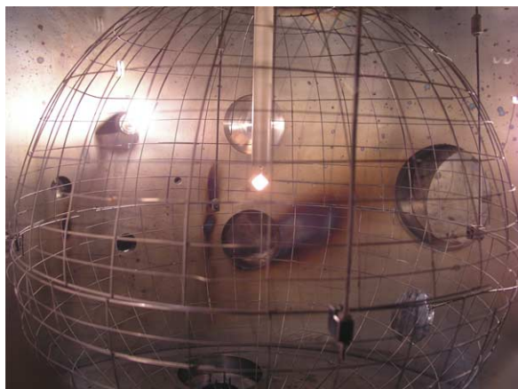
Fig. 4. Tungsten sample during run conditions at 20 kV, 10 mA.
